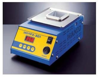
and maintain the temperature of both lead based and lead-free solders. The solder pots are easily changeable to allow use of multiple solder compositions with the same station. The FX-301 comes standard with a 1.87 lb pot and can also accommodate an optional 2.64 lb pot. A timer feature automatically turns off the solder pot after a user selectable time of 10 to 9990 hours
