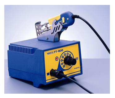
repeatable wire strip lengths from 1-38 mm. To extend the life of the blades the FT-800 has a power save mode. When the FT-8001 handpiece is placed in the holder the station enters the power save mode and reduces the blade temperature by approximately 50%. The FT-8001 handpiece has an indicator light that shows when the blade temperature has stabilized.
