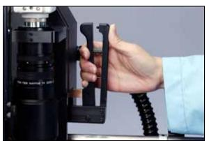
Figure 9: X-Axis Adjust Handle
