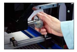
Figure 14: Z-Axis Fine Adjust Knob
