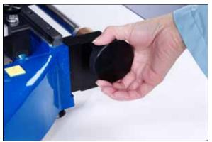
Figure 10: Y-Axis Fine Adjust Knob
