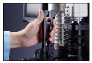
Figure 13: Z-Axis Adjust Handle
