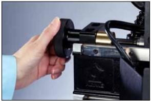
Figure 8: X-Axis Fine Adjust Knob
