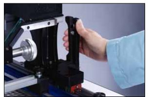
Figure 11: Y-Axis Adjust Handle
