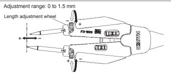
Step 2 Height and the tip end rotation angle
