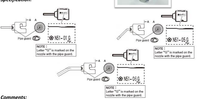
The N51-01, N51-05 and N51-06 nozzles have changed with an upgraded pipe guard that will prevent the use of the vacuum pickup and will prevent damage to the unit. The new nozzles will be denoted on the outside of the nozzle by a "G" following the part number.
