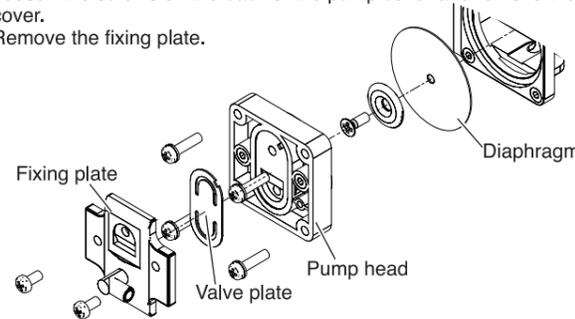
3. Clean the valve plate, fixing plate and pump head with isopropyl alcohol. Align the notch on the pump head with the corresponding notch on the valve plate. Match the notch on the outside of the pump head with the one on the fixing plate. Mount the diaphragm so that it is smooth and taut.
