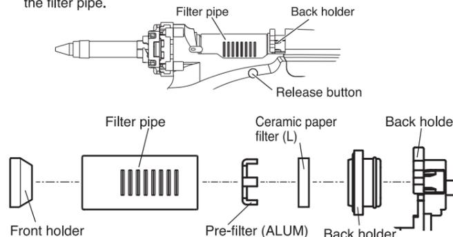
2. Inspect the parts shown in the diagram above. Clean and/or replace as needed.
