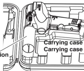
\* Before storing the unit in the carrying case, be sure to insert the nozzle into the protection cover to prevent risk of a burn and melting the carrying case.
