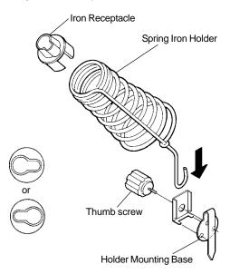
Set the iron receptacle in the spring iron holder keeping the iron tip and the guide pipe horizontally.
