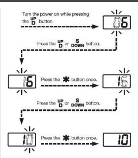
The channel D setting is completed as shown in the preceding diagram. Repeatedly pressing the \*\text{\$\psi}\$ button moves to the channel S setting. (The process is the same as that for channel D.)
