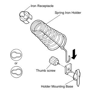
Set the iron receptacle in the spring iron holder keeping the iron tip and the guide pipe horizontally.
