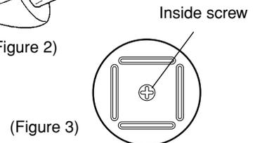
When installing an optional nozzle to the Hakko 850D, do not remove this inside screw.
