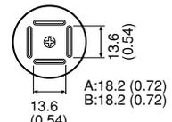
**A1181B** BQFP 19 x 19 (0.75 x 0.75)      **A1182B** BQFP 24 x 24 (0.94 x 0.94)      **A1183** SOJ 15 x 8 (0.59 x 0.31)      **A1184B** SOJ 18 x 8 (0.71 x 0.31)      **A1185B** TSOL 13 x 10 (0.51 x 0.39)
